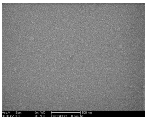
Figure 117: SEM analysis of Au doped \text{TiO}_2 film, 400 °C
