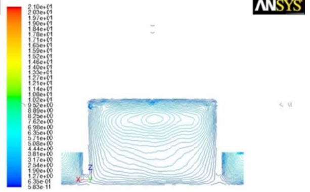
Contours of Turbulent Kinetic Energy (k) (m2/s2)
