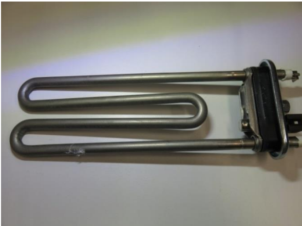
Figure 22: Abrasion observed on the heating element of Device E during the final inspection
