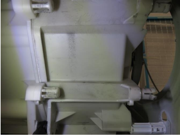
Figure 21: Grey layer observed on the front drum ring of Device E
