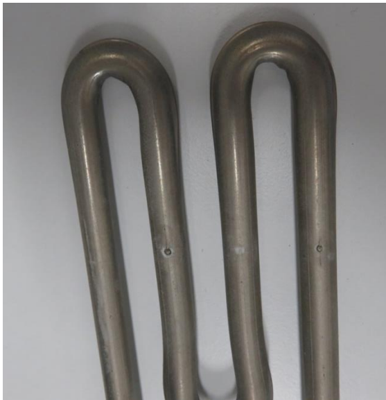
Figure 20: Abrasion observed on the heating element of Device D during the final inspection
