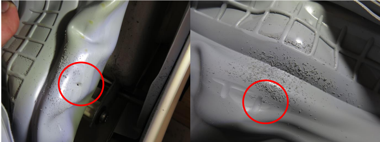
Figure 19: Abrasion and hole observed on the door gasket of Device D during the final inspection
