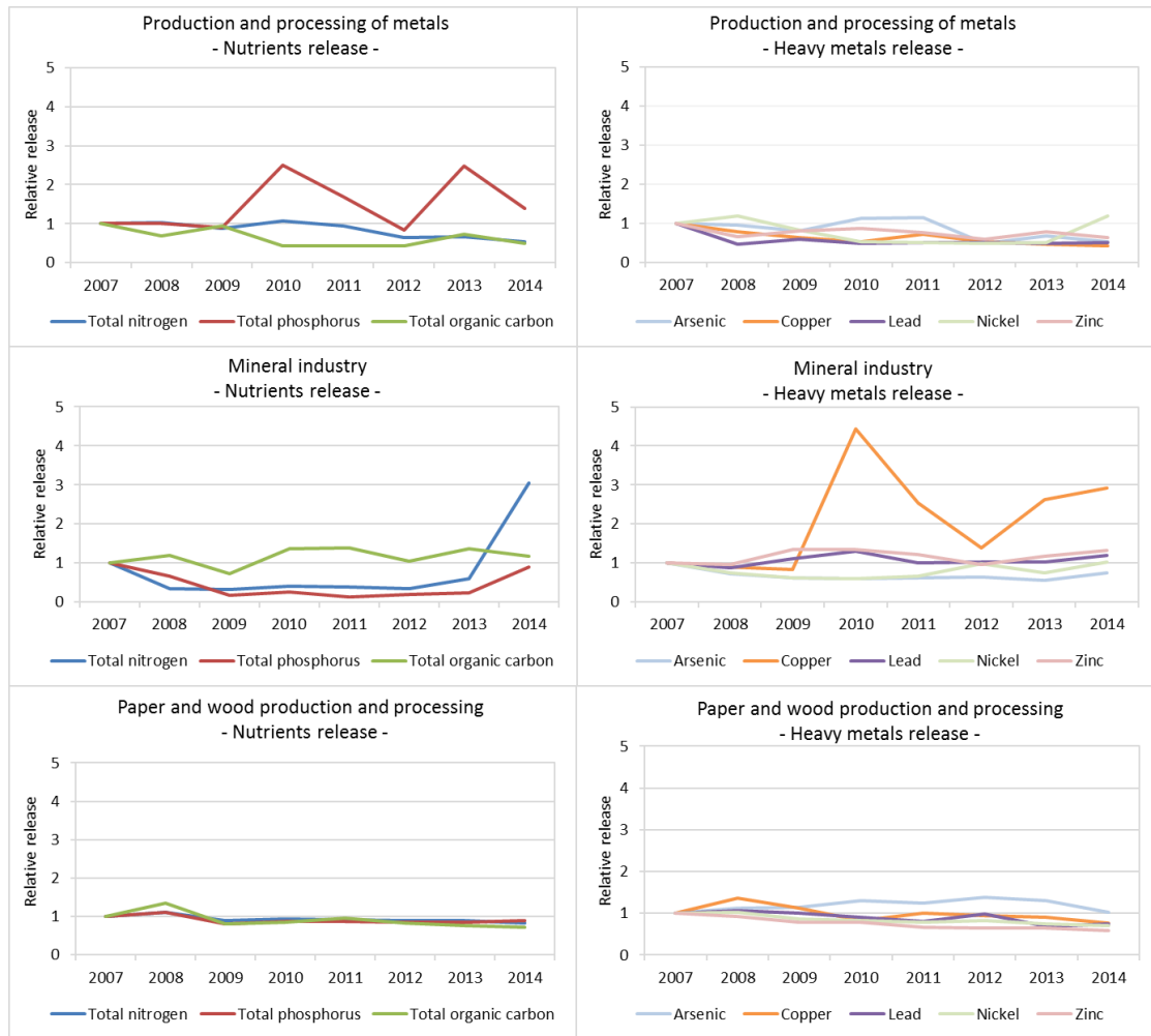
Figure 6: Release of pollutants from the metals, minerals, paper and wood industries (17) over the period 2007-2014 according to E-PRTR data. Data refer to values relative to 2007 and cover the eight most reported pollutants in E-PRTR.
