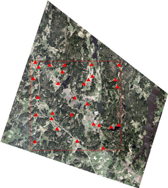
Figure 8 ICPs datasets used by JRC over chosen LPIS QA 2016 SE-3-2 site to calculate the relative geometric accuracy of PlanetScope ortho imagery (overlay on WV2 orthoimage).
