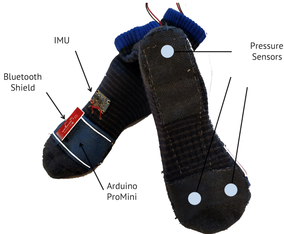
Figure 5-11: Design of the SoPhy socks: The socks have sensors attached to the sole and bridge of the foot to capture lower body movements of the patients.
