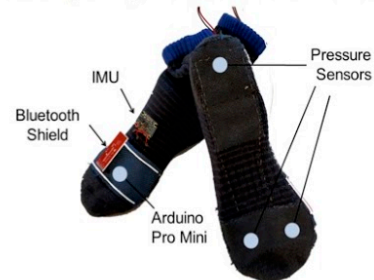
Figure 1: The wearable components of SoPhy : Each sock consists of three pressure sensors and one IMU.
