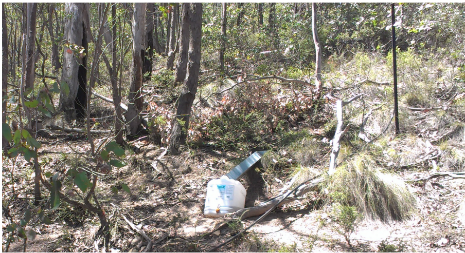
Figure 4.1: Example of throughfall trough installation, illustrating the slope effect on the trough surface area.
