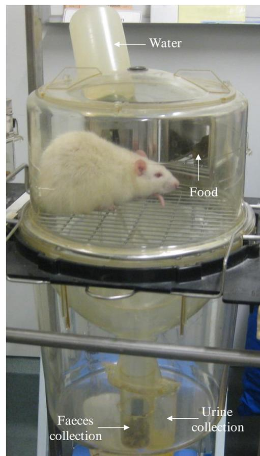
**Figure 2.5 Metabolic cage set-up**
