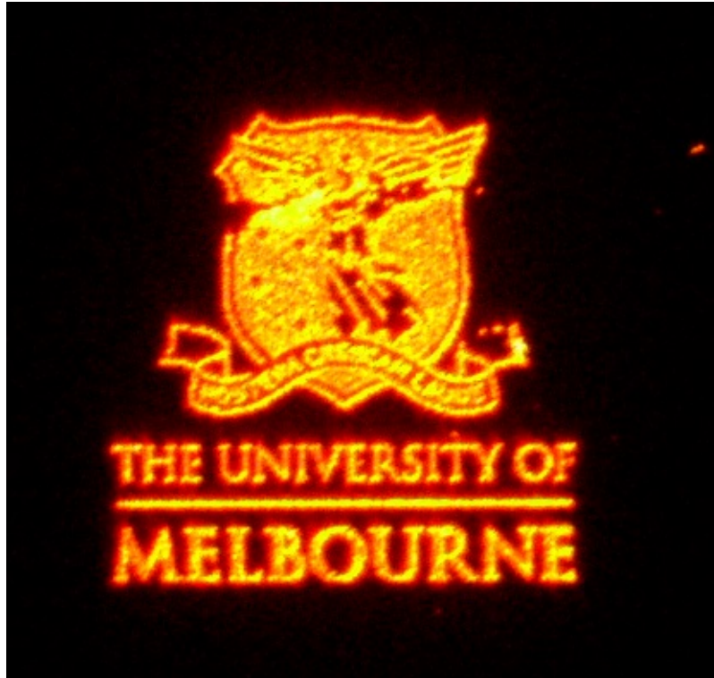
Figure 1.8: A darkfield microscope image of a plasmonic array of nanocavities fabricated using RNIL.
