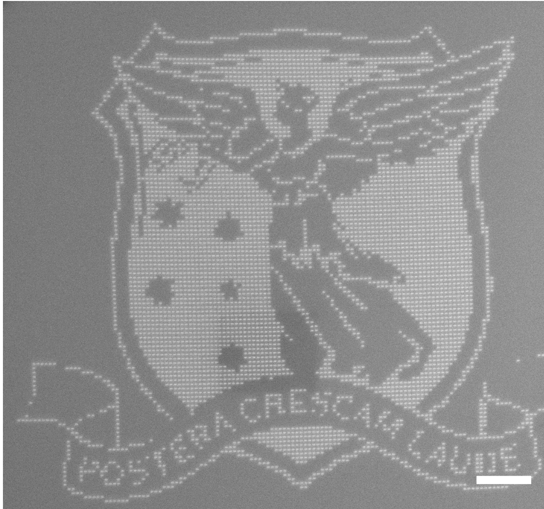
Figure 6.14: An SEM image of a HSQ/Si master template, consisting of a structured array of 200 nm by 50 nm nanorods. The white scale bar is 5 \mu\text{m} . The image has been reversed.
