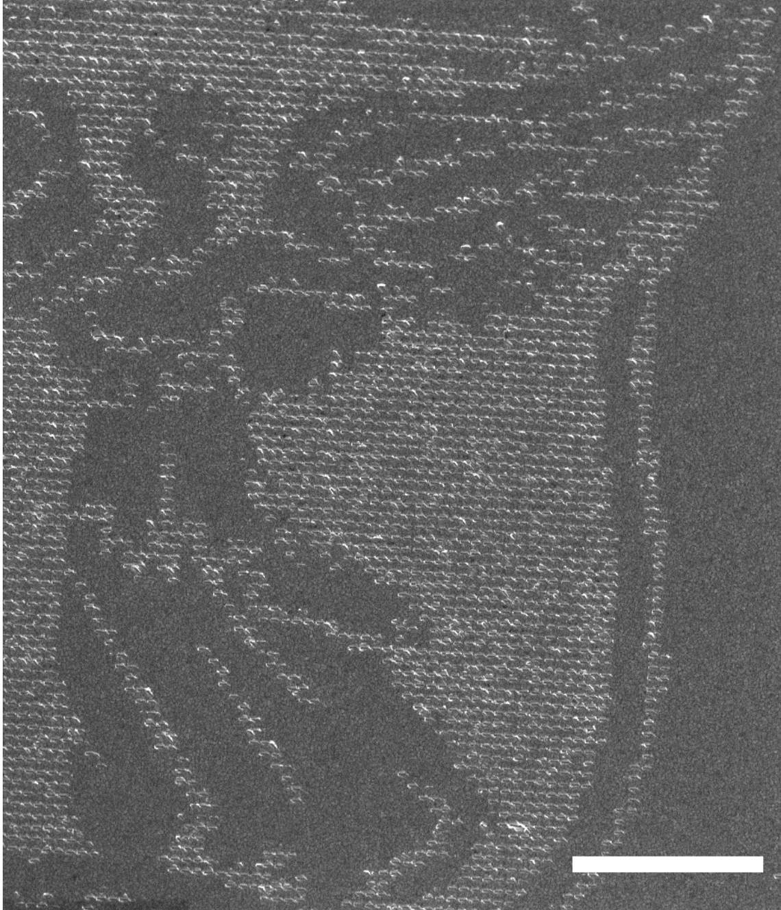
Figure 6.15: An SEM image of the imprint in a silver film produced using the master shown in Fig. 6.14. Note the fine details are made up of only a few nanocavities. The white scale bar is 5 \mu\text{m}
