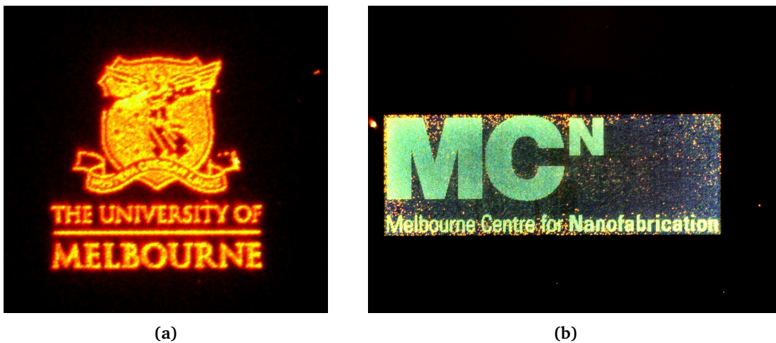
Figure 6.18: Darkfield microscope images of the University Crest metasurface imprinted into a thin silver film (a) and the MCN logo metasurface imprinted into a thin silver film (b). The nanocavities comprising the metasurfaces are the same dimensions.
