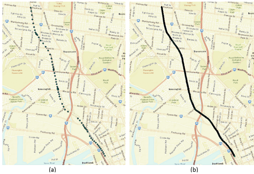
Figure 39: A raw trajectory with occasional signal loss (a), an interpolated smoothed trajectory after linear interpolation (b).
