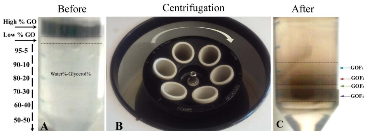
Figure 3-3. Separation of GO nano sheets using glycerol density gradient
