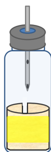
Figure 4 A 20-ml, crimp-cap headspace vial with a sample of watercolour on paper. After degradation in the sealed vial, the sample is loaded into the HT3 and analysed by P&T-HS-GC-MS.
