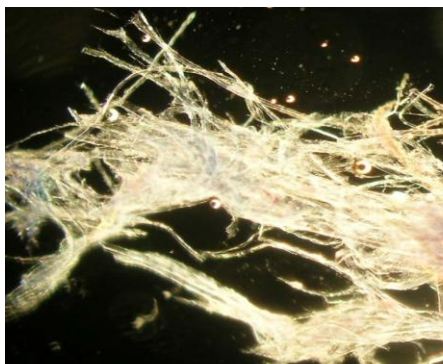
Figure 1 A fibre sample stained with neocarmine, dark field, and 40 x. The fibres are quite disrupted and identification by structural features alone is difficult, but by adding neocarmine W it is possible to note that most of the fibres are flax, reddish, with a few cotton fibres, blue, also present. The fibre ratio was variable between slides, but ca. 50:1 flax/cotton is typical. Also visible in the upper right is a wool fibre that is stained yellow by the neocarmine W.
