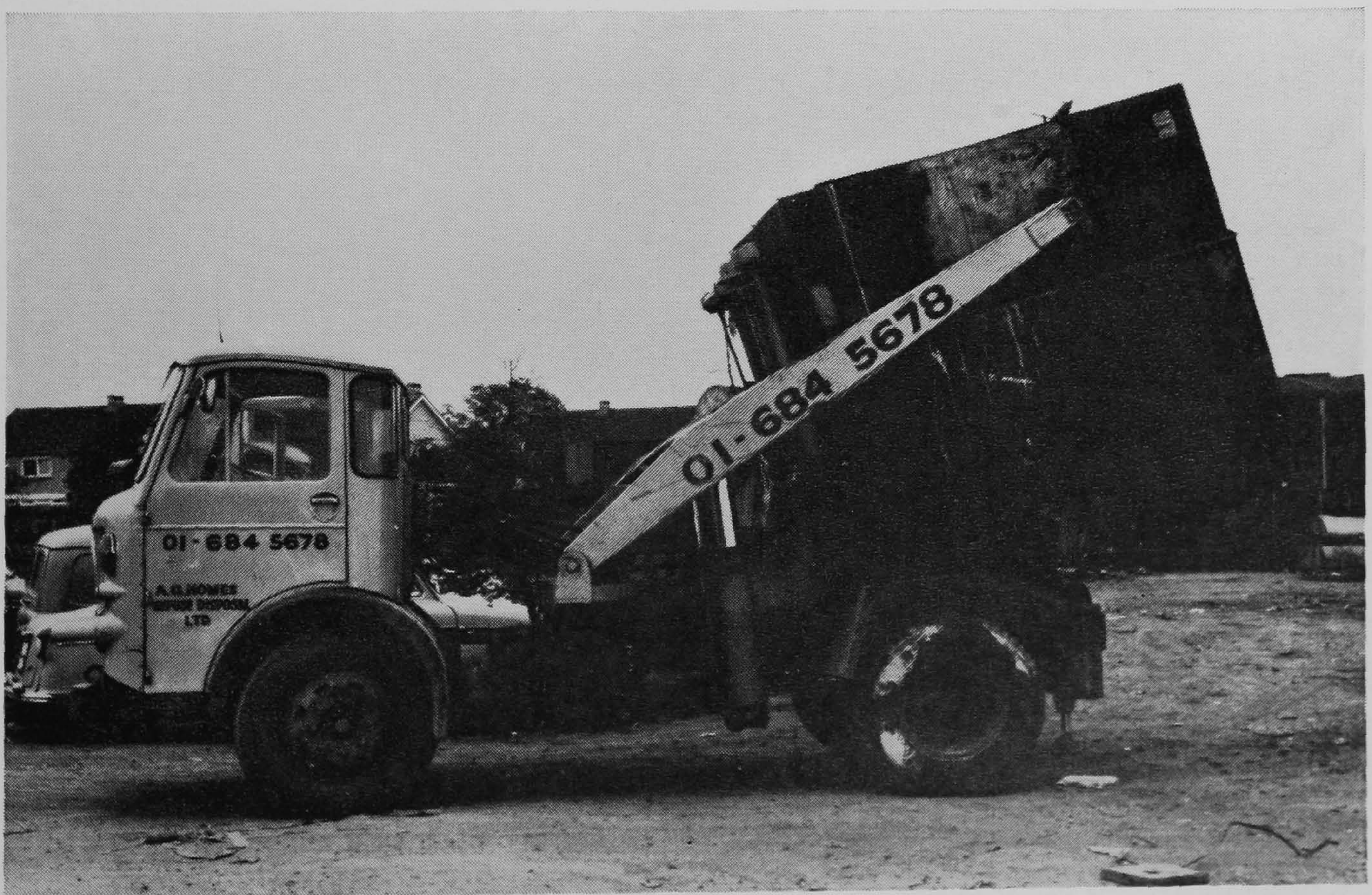
Showing length of free chain when arms are in a low position.
