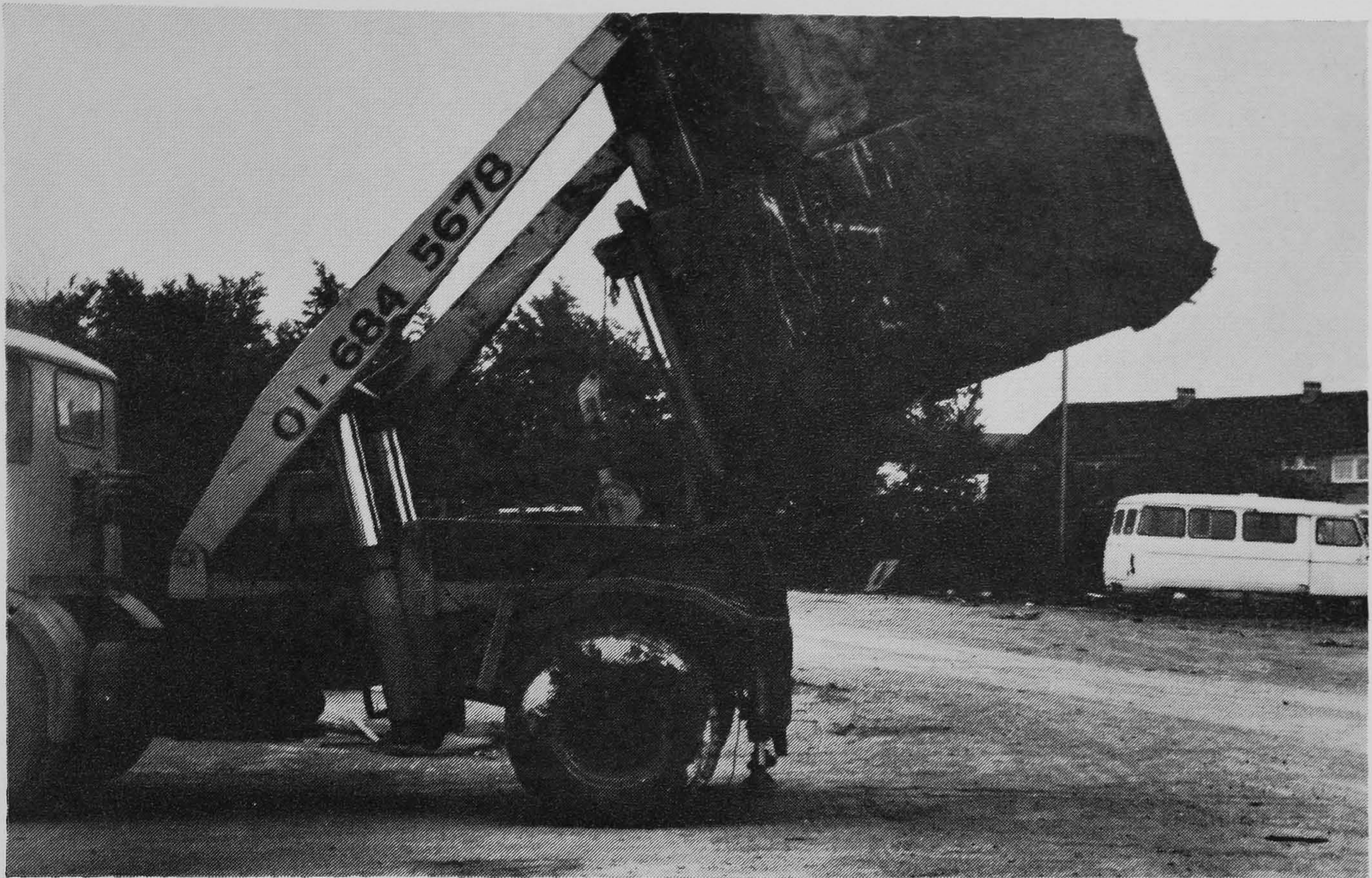
Illustrating "Demonstration unloading" with arms in high position and chains taunt. Note:—Weight of container is supported by chains and lowered against backrest of lorry.
