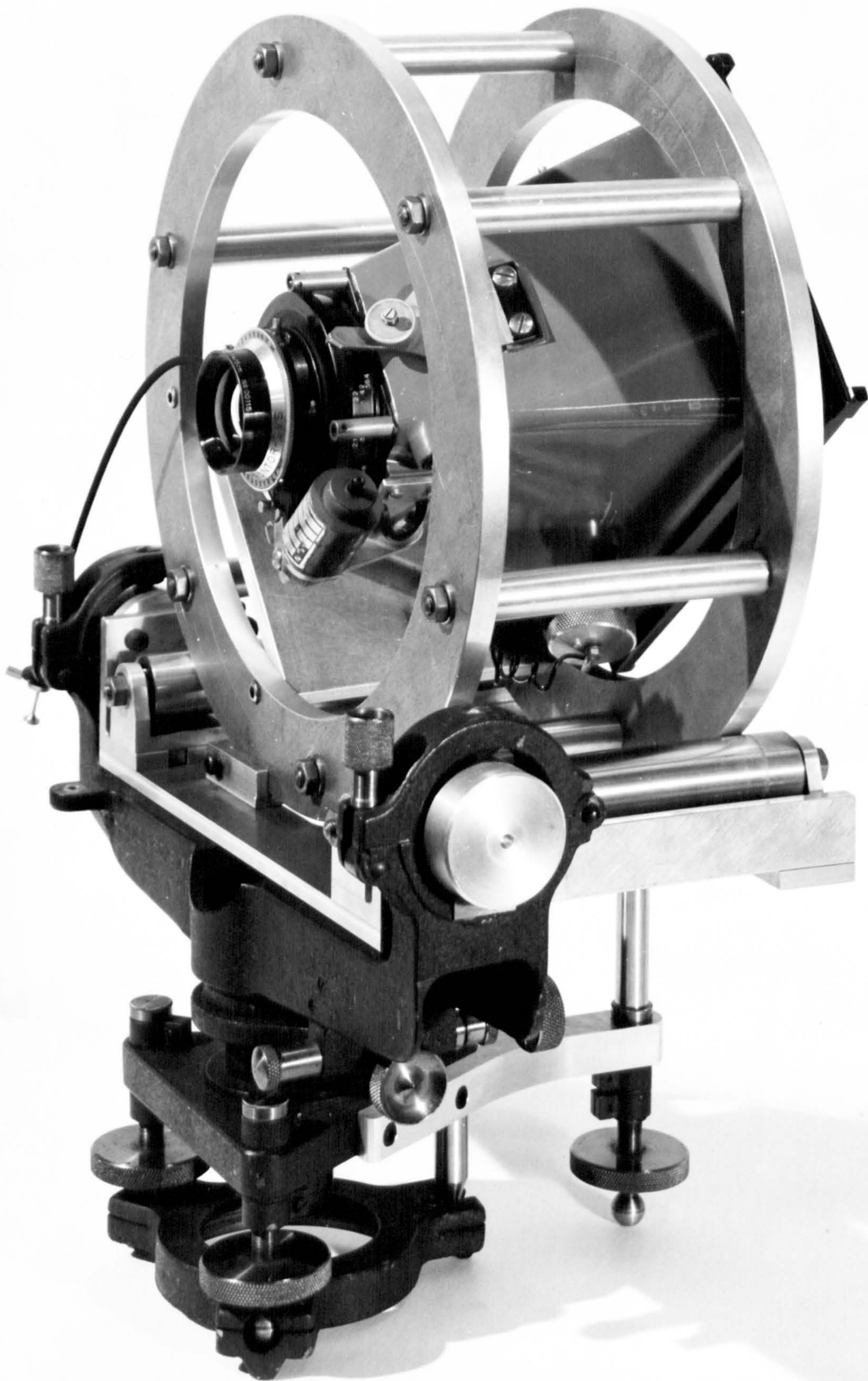
Plate 8. The camera, cage, roller assembly and tribrach. Note the extended rear footscrew.
