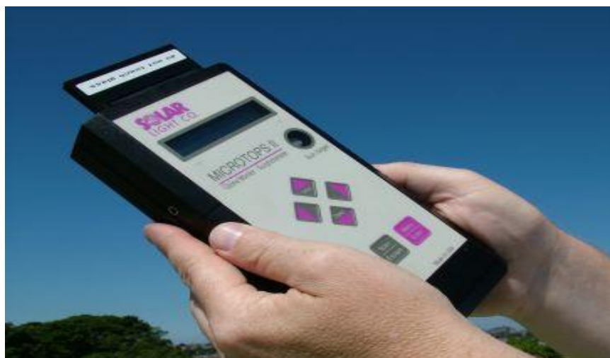
Figure B: Microtops II sunphotometer with sun target and GPS attachment. Photograph courtesy of NERC Field Spectroscopy Facility.
