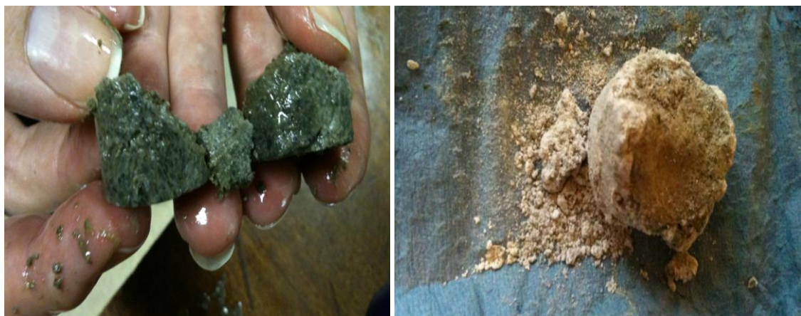
Figure 8.8: Photographs of the natrocarbonatite core sample used for permeability tests. (a) Directly after removal from the permeameter where sample has broken in half with alteration occurring; (b) 24 hours after the permeability test sample has dried to brown, unconsolidated, altered unit.
