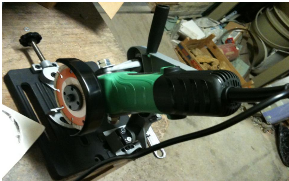
Figure 2.1: Bench mounted angle grinder used to cut samples containing hygroscopic material. Blade diameter 11.5cm and diamond coated.
