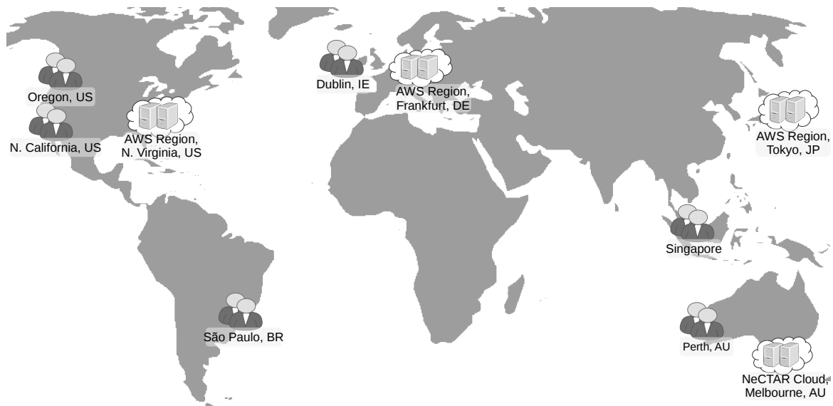
Figure 6.6: Experiment 1 — 4 cloud sites host the Entry Points and Admission Controllers ; 6 cloud sites are used to emulate incoming users.
