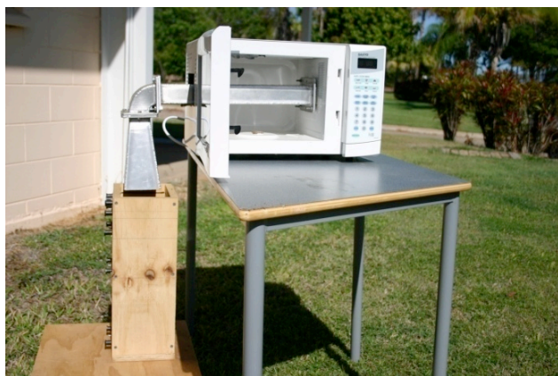
Figure 3: Microwave prototype system based on a modified microwave oven.
