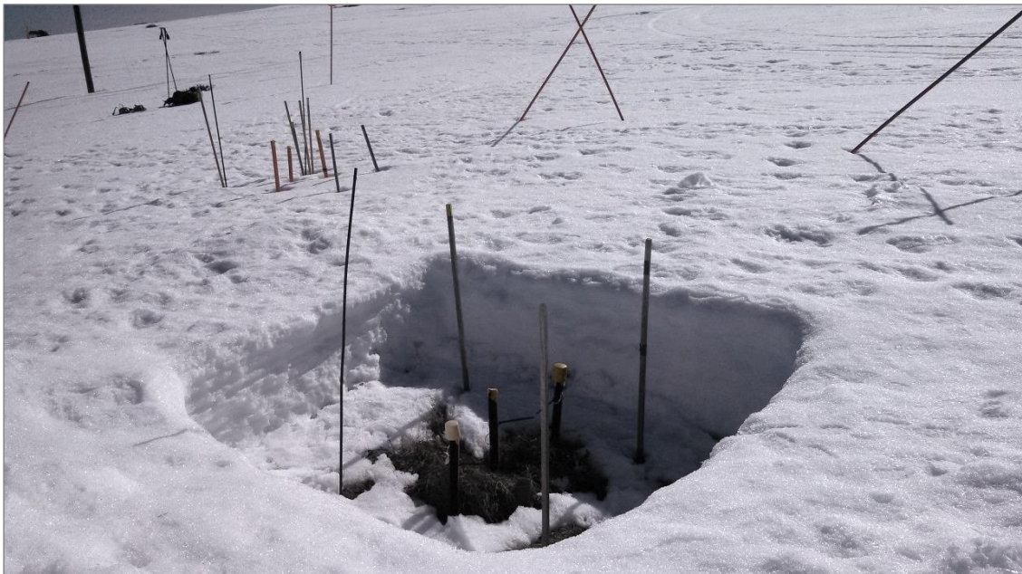
Figure 7.6. Experimental manipulation of snow depth. Experimental snow removal plots (front) were kept clear of snow throughout the winter while control plots (rear) accumulated snow naturally.
