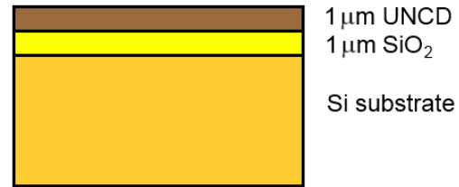
Figure 4.3: Structure of the substrate wafer used for N-UNCD processing.
