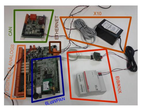
Figure 11. Multi-protocol card used for the evaluation.
