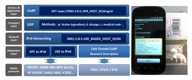
This reads the tag, which contains extended information in link format, such as for CoAP; this information is accessible through the IPv6 address by mapping the 40 bits from the UID into the host ID
