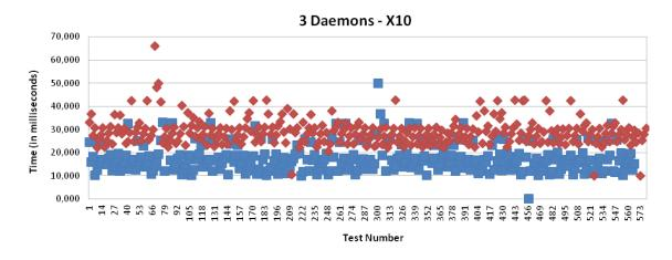
**Figure 19.** Transmission and processing time for CAN technology with mapping (red) and without mapping (blue), when three daemons are managing the requests.
