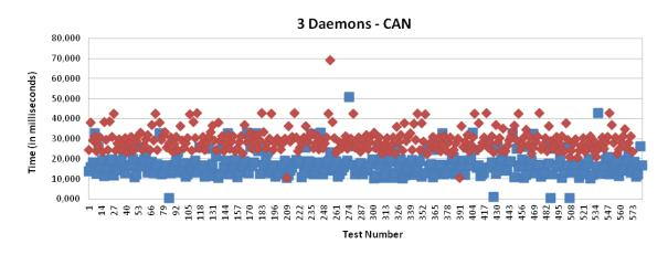
**Figure 20.** Transmission and processing time for EIB/KNX technology with mapping (red) and without mapping (blue), when three daemons are managing the requests.
