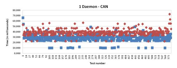
**Figure 17.** Transmission and processing time for EIB/KNX technology with mapping (red) and without mapping (blue), when a single daemon is managing all the requests.
