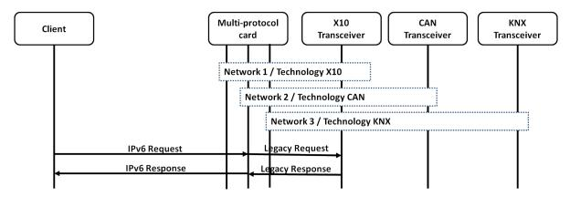
Figure 14. Evaluation environment with a daemon and interface per technology.
