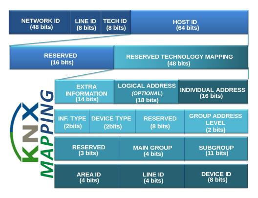
Figure 6. Full mapping from host ID to the EIB/KNX address.
