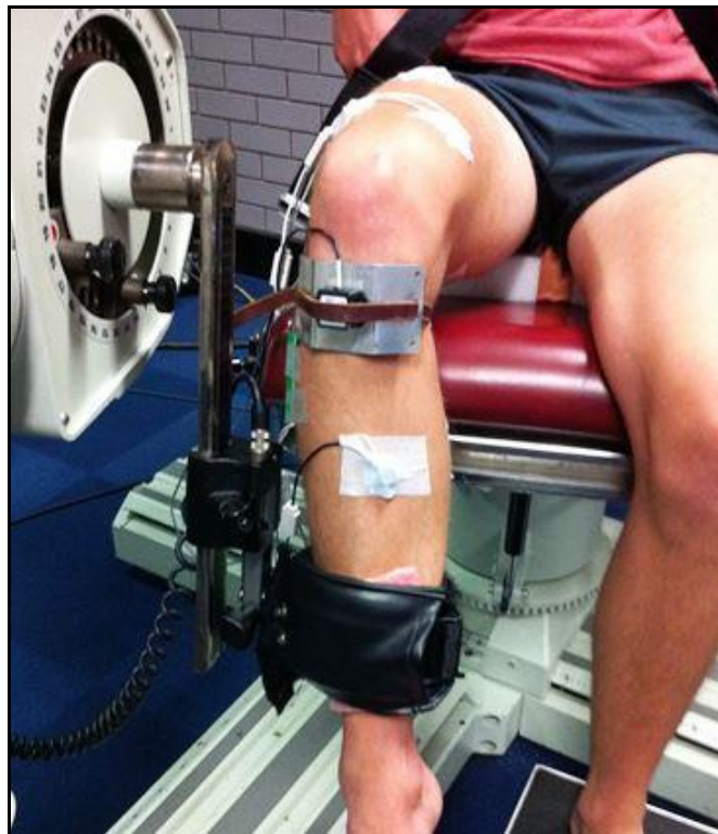
Figure 4.2. Isometric testing position with participants seated on a foam platform on the seat of a KinCom isokinetic dynamometer with the thigh elevated.
