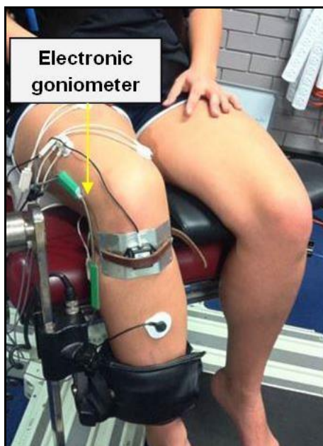
Figure 4.4a. The electronic goniometer that was used to monitor knee flexion angle during testing
