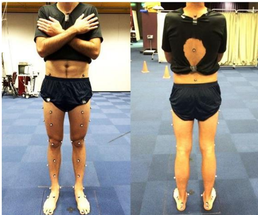
Figure 5.1 Locations of the 40 retro-reflective markers on the trunk, pelvis, thighs, legs and feet of a participant. The exact anatomical locations and orientations of each marker are provided in Appendix 9.
