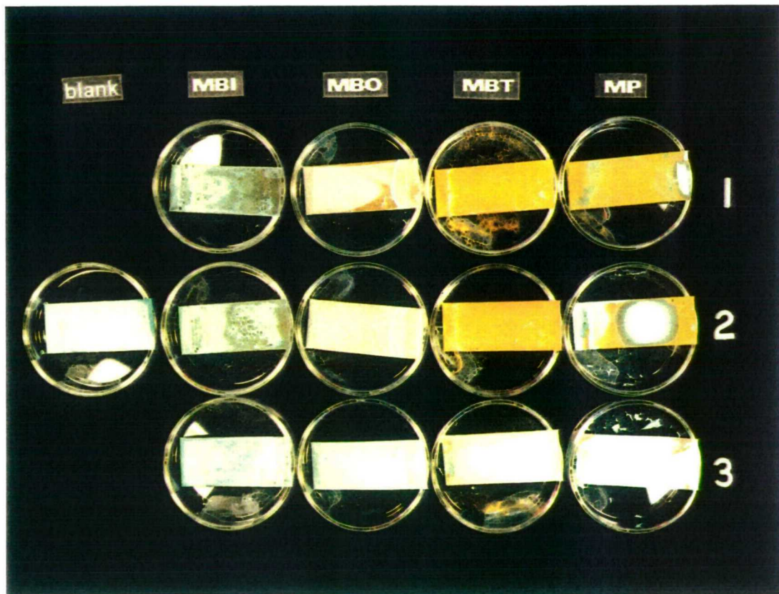
Figure 5. 3 Coupons after 24 hours at 95% RH Ambient Temperature.
