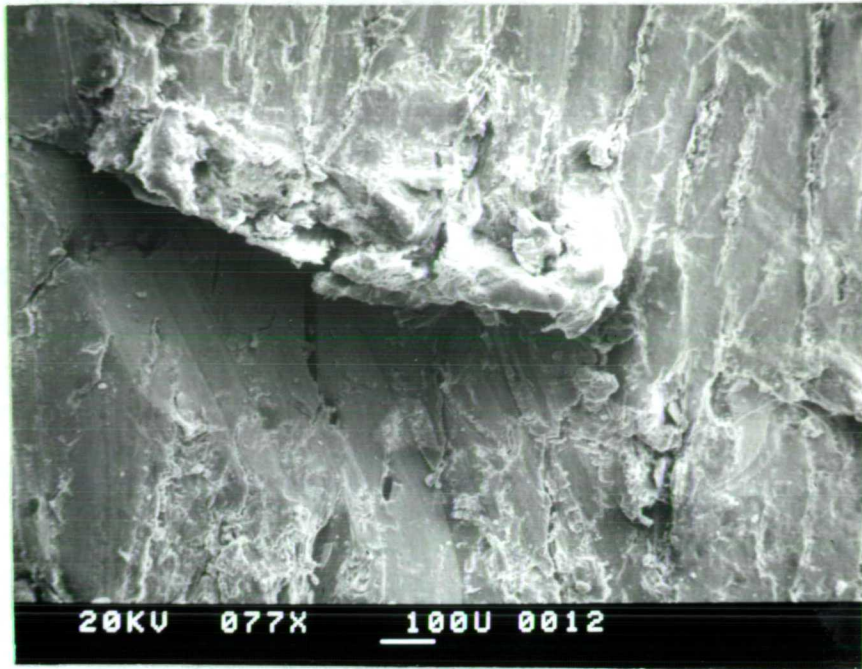
Fig. 43 Same flaker showing amasssed debris at terminus of one of the striations (77X).
