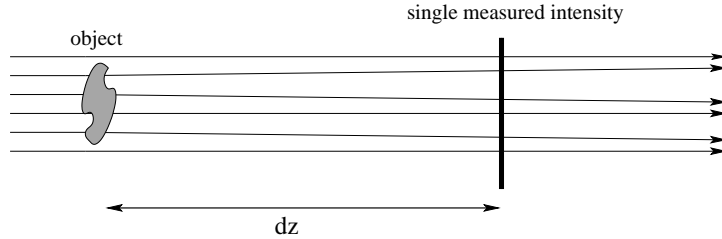
Figure 2.16: Configuration for applying single plane TIE based phase retrieval algorithm. The measured intensities have a distance dz from the object.
