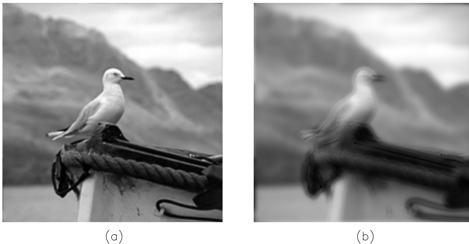
Figure 4.17: Phase retrieval in a noise free environment for (a) small propagation distance z_2 = 0.03m , phase retrieval is perfect for the whole frequency spectrum, and (b) larger distance z_2 = 0.63m , the source blurring influences phase retrieval.
