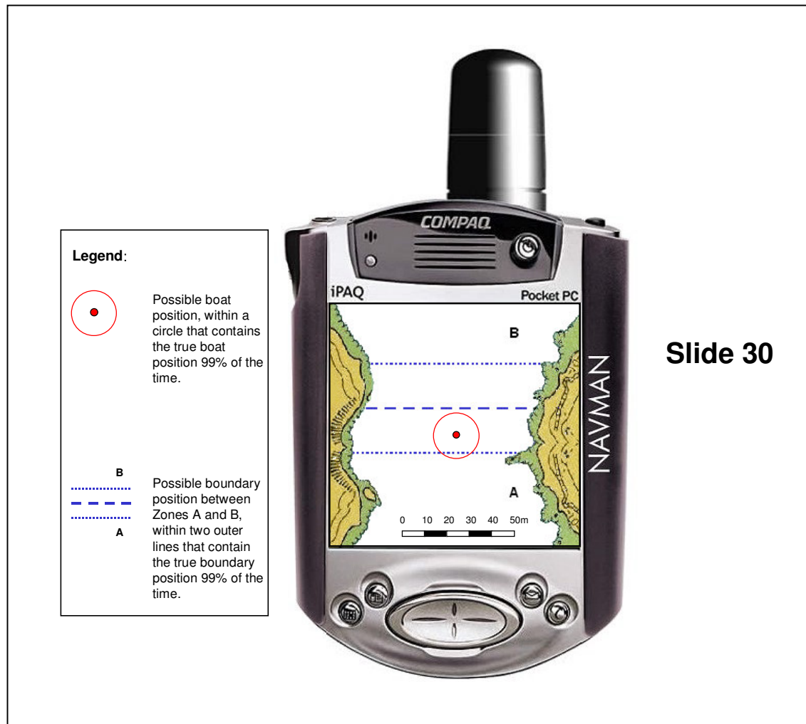
Figure 4.3. Example slide showing the Limits representation of positional uncertainty in the navigation case study.
