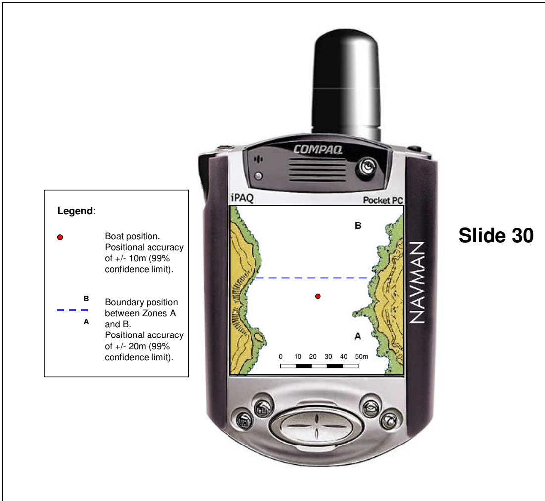
Figure 4.4. Example slide showing the Scale representation of positional uncertainty in the navigation case study.
