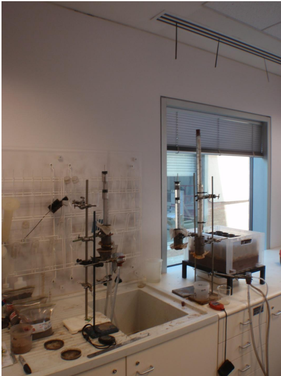
Figure 1. Mini-disc infiltrimeters and soil cores held in place using a clamp and stand. A buchner funnel was used to create a negative pressure at the bottom of the core (this can be seen in the clamp and stand positioned to the left of the basin). The cores were placed in the tension table (far right hand side) between infiltration experiments in order to (eventually) obtain saturated soil cores.
