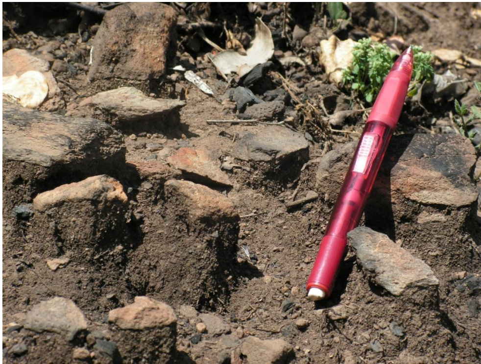
Figure 9. Intact pedestals used to obtain a measure of erosion depth on hillslopes. Photo is from Yarrarabula in November 2007.
