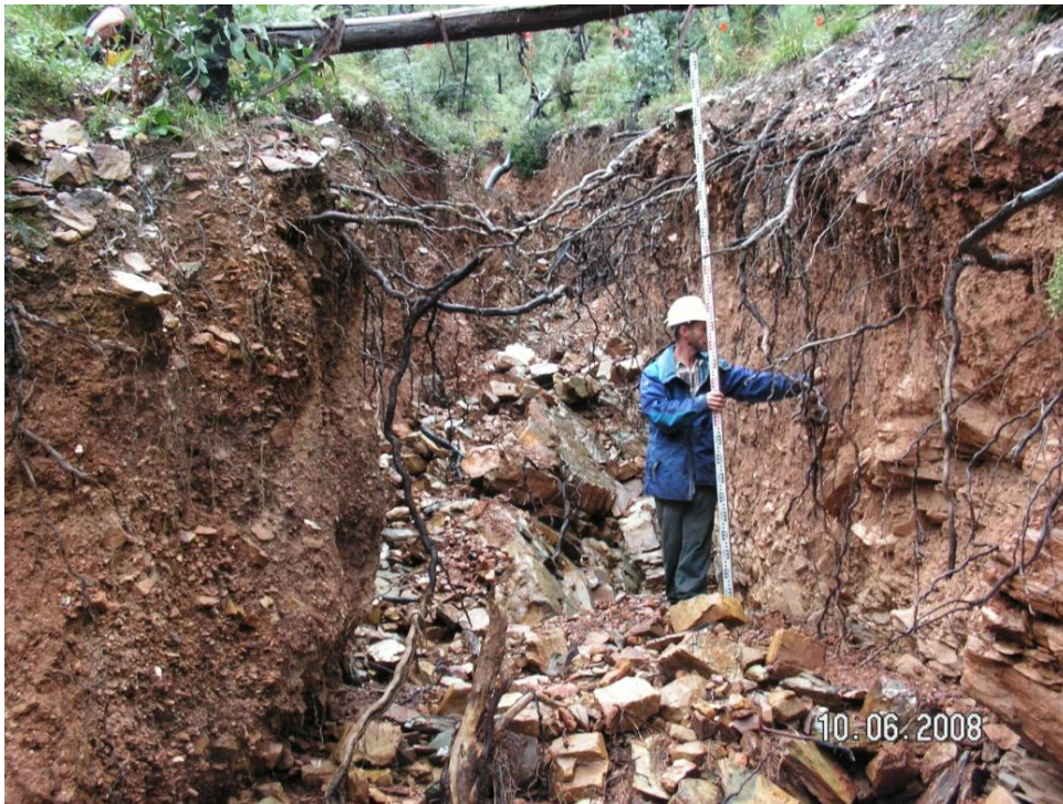
Figure 7. Measuring channel cross sections in headwaters of Rose River that were scoured by debris flows in December 2007
