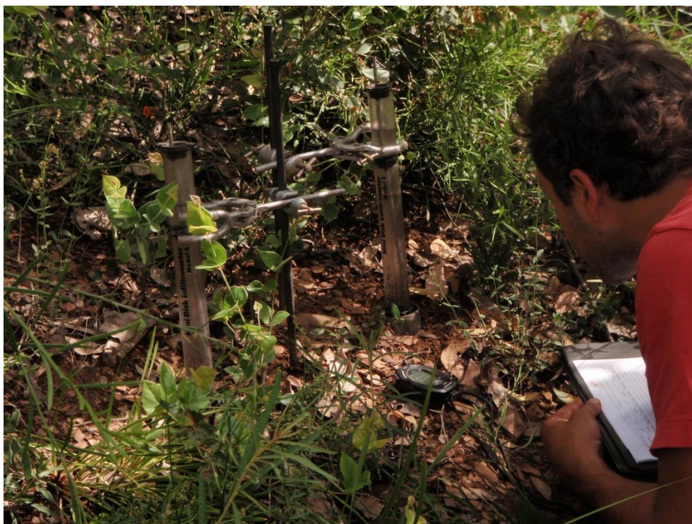
Figure 2. Using min-disc infiltrometers from Decagon to measure infiltration rates at Ella Creek, 3 years after wildfire. Peter Mercurio is carefully taking a reading.
