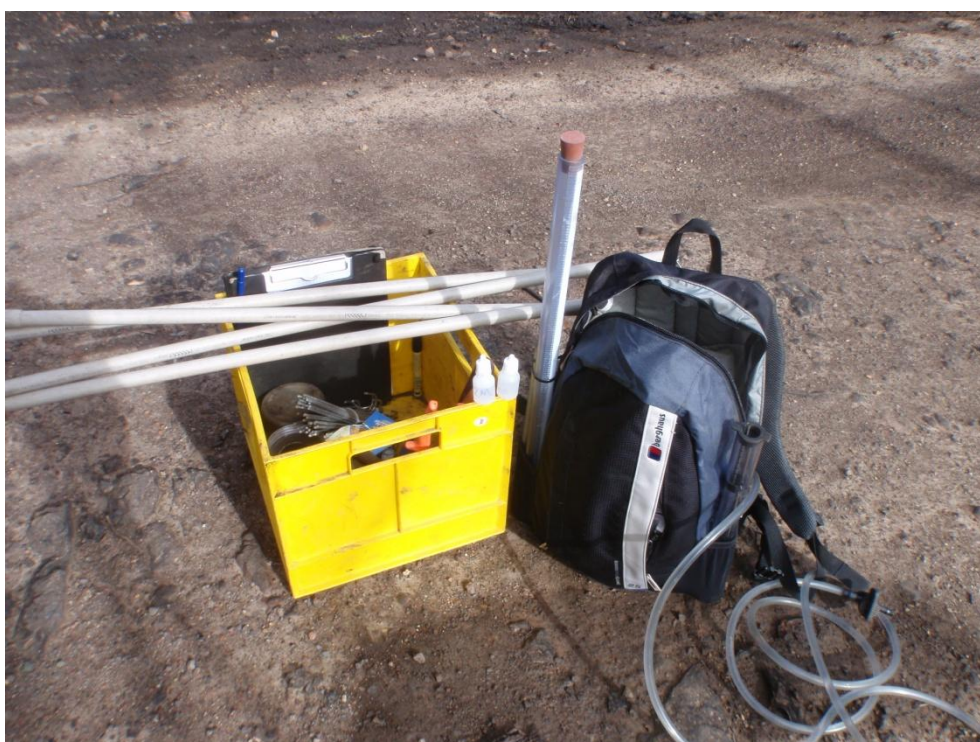
Figure 3. Infiltrometers require little water and are easily carried around headwaters enabling widespread sampling of infiltration properties. Water was carried in a 15 L bladder inside the backpack.
