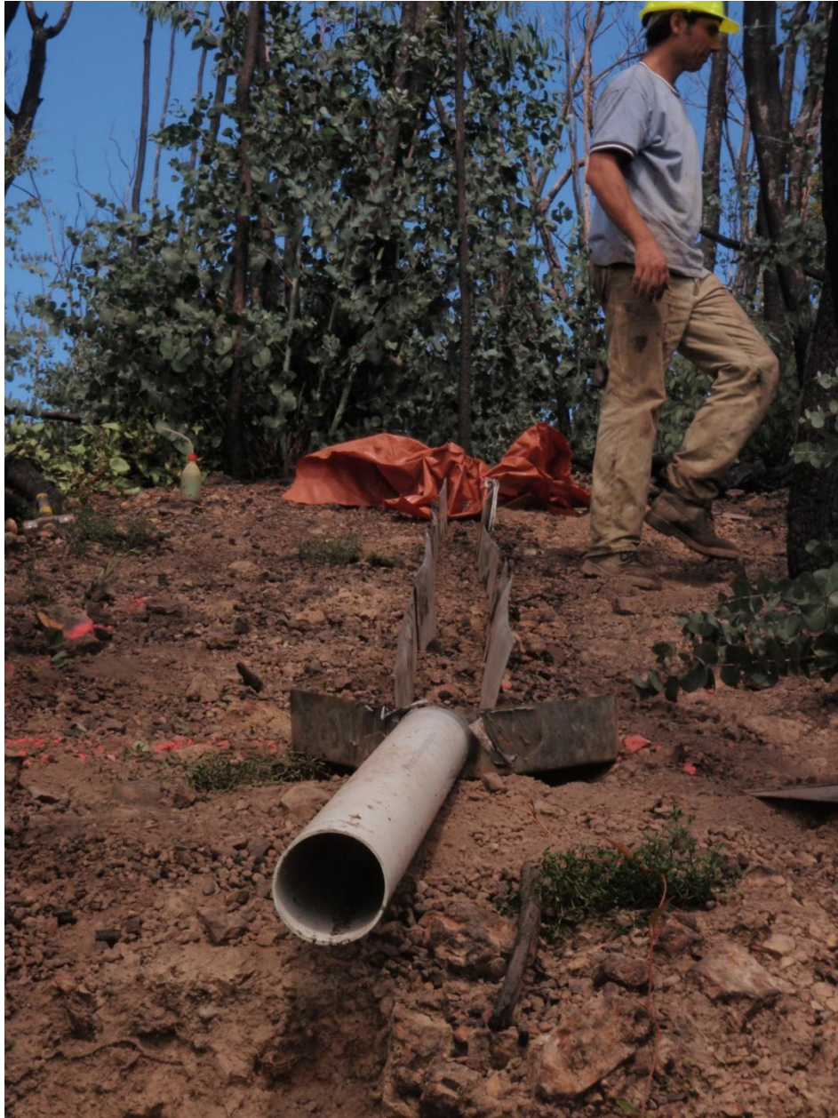
Figure 4. Flume experiments on hillslopes at Sunday Creek. Water was pumped through a rotameter and introduced to the test area from a small retention basin at the top of the flume. The test area is 4 m long and 0.15 m wide. Sediment was collected at the pipe outlet in 0.5 L containers at set time intervals. Philip Noske is walking off to start the pump.
