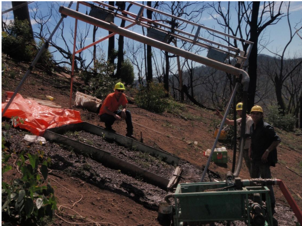
Figure 5. Rainfall simulation setup on steep slopes ( 25^\circ ) at Sunday Creek. With help from Sina Moshirvaziri, Craig Mason and Gary Sheridan.
