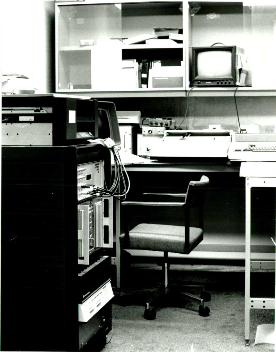
figure 4.1 Photograph of the minicomputer based experimental OAE measurement instrument. The main components are a 16bit minicomputer, a Cambridge Electronic Design analogue interface and an 80MByte winchester disk.
