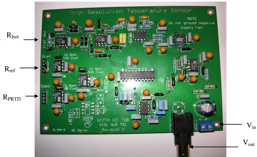
Figure 2.32. Photograph of high resolution temperature measurement device indicating voltage input, measurement output, current setting resistor, sense resistor and PRTD attachment.
