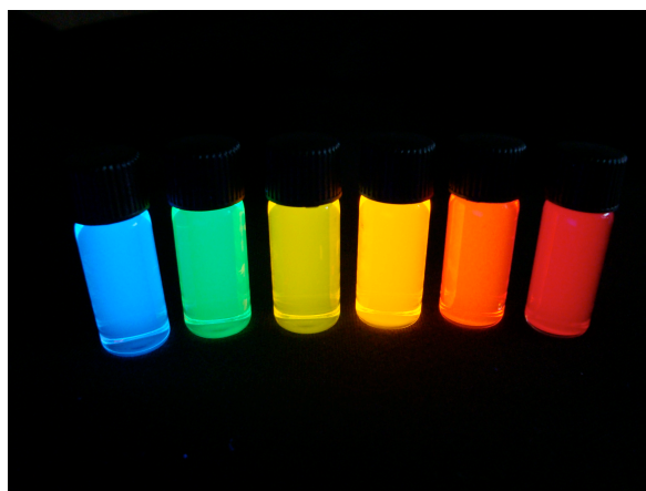
Figure 2.3 Series of CdSe quantum dots dispersed in chloroform illuminated under low power UV-light. Emission wavelengths spanning the entire visible spectrum are realised through size-tunable synthetic schemes. Image courtesy of T.-L. Nguyen.
