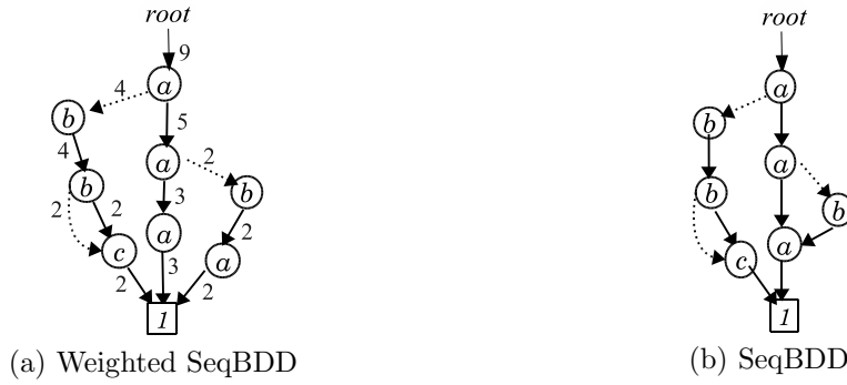
Figure 5.4: Weighted SeqBDD vs SeqBDD for a set of sequences S = \{aaa : 3, aba : 2, bc : 2, bbc : 2\} , using a lexicographic variable ordering
