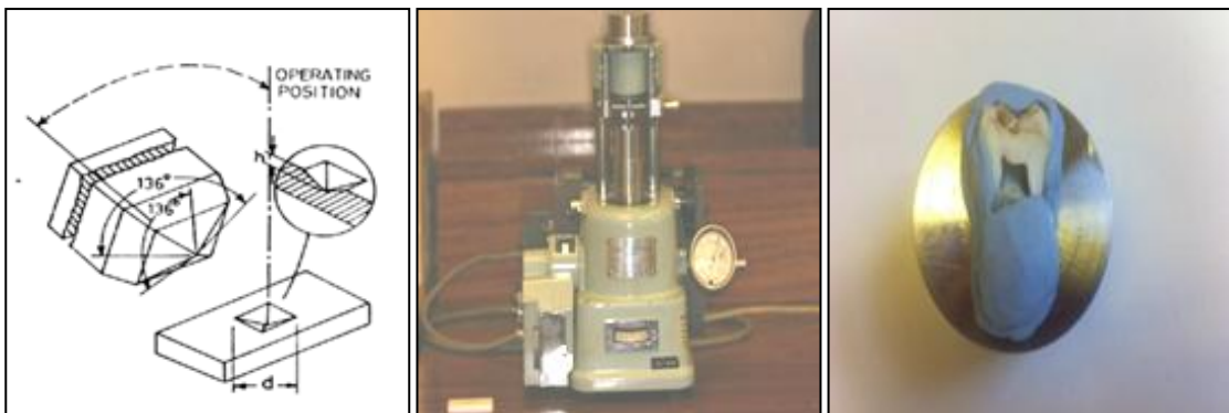
Figure 3.8: Wallace indenter is an instrument used to measure hardness. Stabilization of the teeth using a reusable putty-like pressure-sensitive adhesive around the tooth surface only but not between the tooth and the sample plate of the Wallace.
