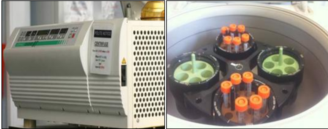
Figure 3.14: High centrifuging force can minimize the amount of the turbid material that can be present in the purified DNA
