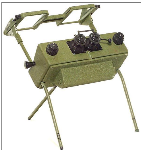
Figura 104- Old Delft Scanning Stereoscope III.
