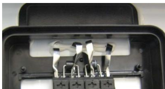
Figure 3.16 – Delamination can cause these ribbons to open and get in short-circuit [Zgonena, 2010].
