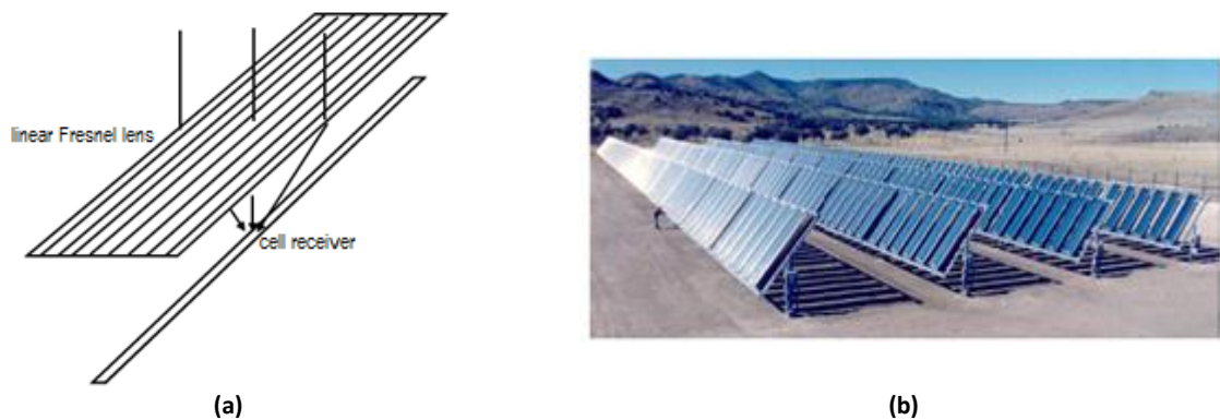
Figure 2.6 – Concentrator systems with refractive optical elements a) Linear Fresnel lens concentrator concept. b) Entech™ 100 kW PV power plant [Spinoff, 2002].
