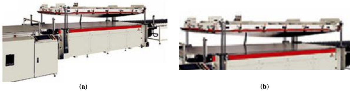
Figure 3.2 – a) Spire vacuum laminator where lower and upper chambers are visible. b) Enlargement of upper and lower chambers in the Spire vacuum laminator [Spire Solar, 2010].
