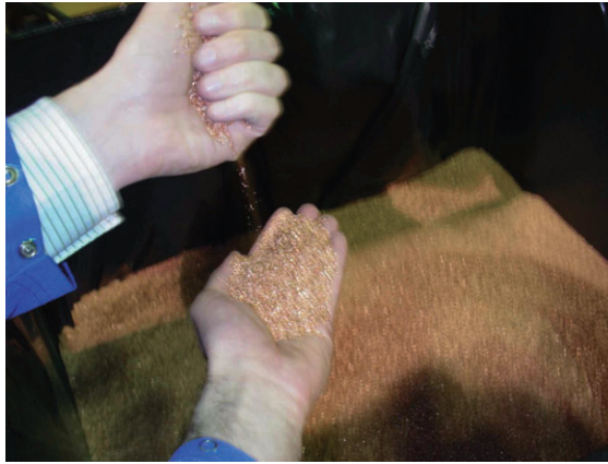
Plate 2 Former e-waste processed into commodity grade copper
