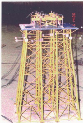
Figure 3.2 Typical Jacket Structure Model
