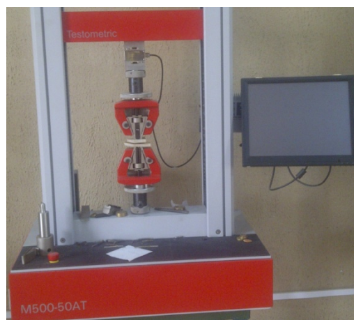
Figure 2. Instron-universal tensile testing machine (M500-50AT)
