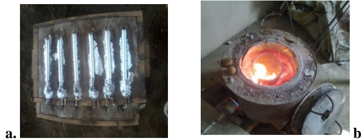
Figure 1. (a) and (b) showing as-cast samples and gas-fired crucible furnace respectively
