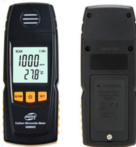
Plate 3.1 Benetech Carbon Monoxide Meter GM8805
