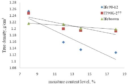
Fig. 2: Effect of moisture content on true density of three cowpea varieties
