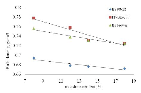
Fig. 1: Effect of moisture content on the bulk densities of three cowpea varieties
