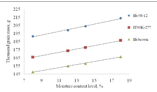
Fig. 3: Effect of moisture content on thousand grain mass of three cowpea varieties
