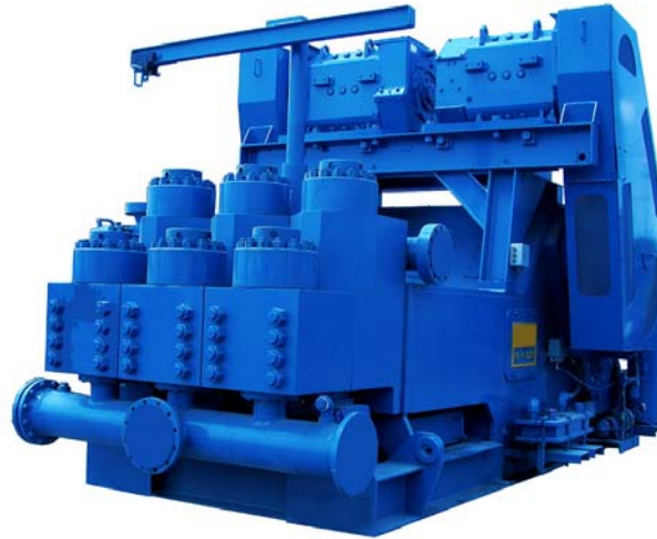
Figure 7 – A three-piston (triplex) mud pump system [43]
