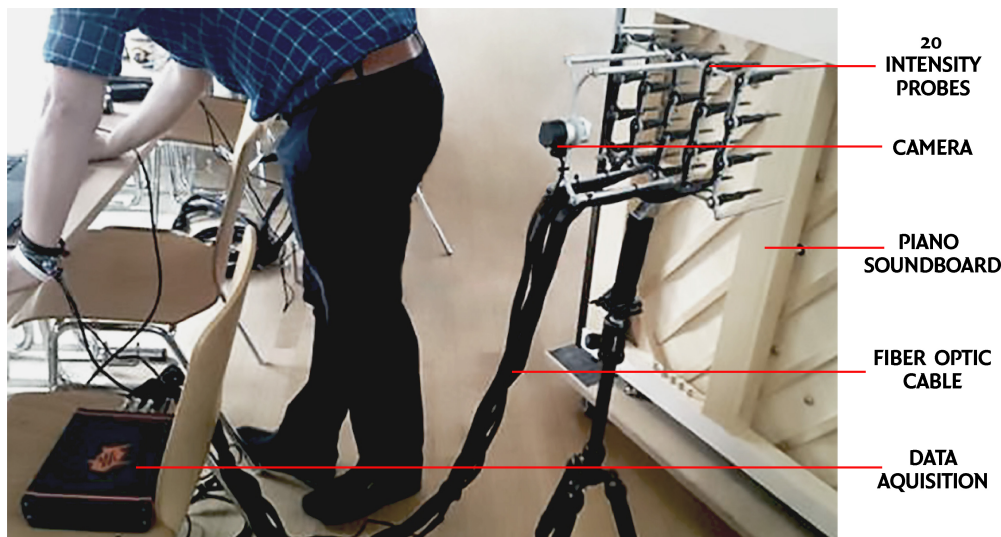
Figure 10: Experimental setup of the acoustic measurements on the piano soundboard using a handheld intensity array.
