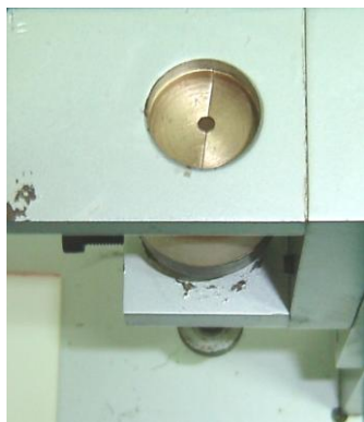
Figure 1: The hole in the brass mould adapted to the bending jig
