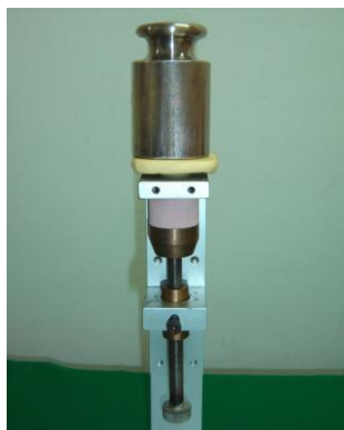
Figure 2: Load application during bonding
