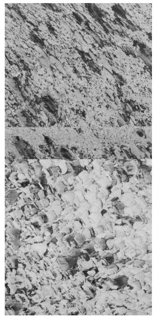
Figure 4: Untreated control surface Figure 5. Surface treated with coca-cola for 5 minutes
