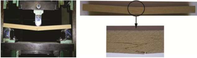
Figure 2: Failure mode of the test specimens for determination of bending strength and modulus of elasticity in bending of tested MDF panels
