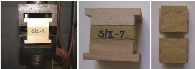
Figure 3: Failure mode of the test specimens for determination of internal bond of tested MDF panels
