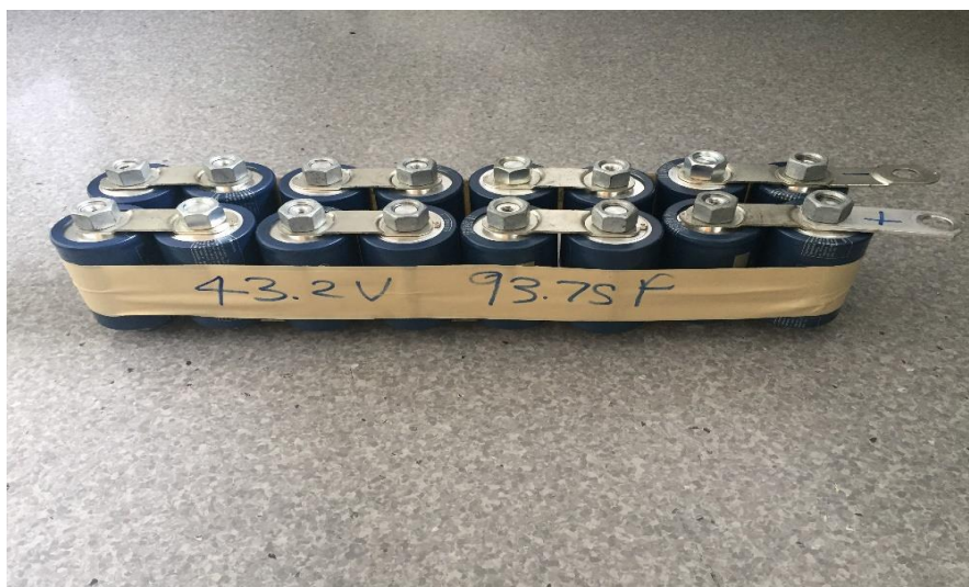
Figure 4-9: SC bank assembled using 16 SCs, each of 2.7 V, 1500 F.
