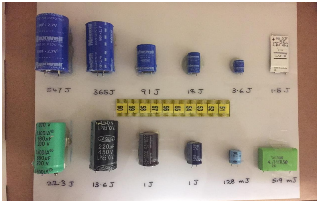
Figure 2-1: Comparison of SCs and electrolytic capacitors in terms of energy and sizes
