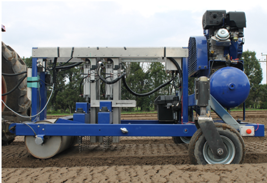
Figure 1.9: Robotic dibbler during testing
