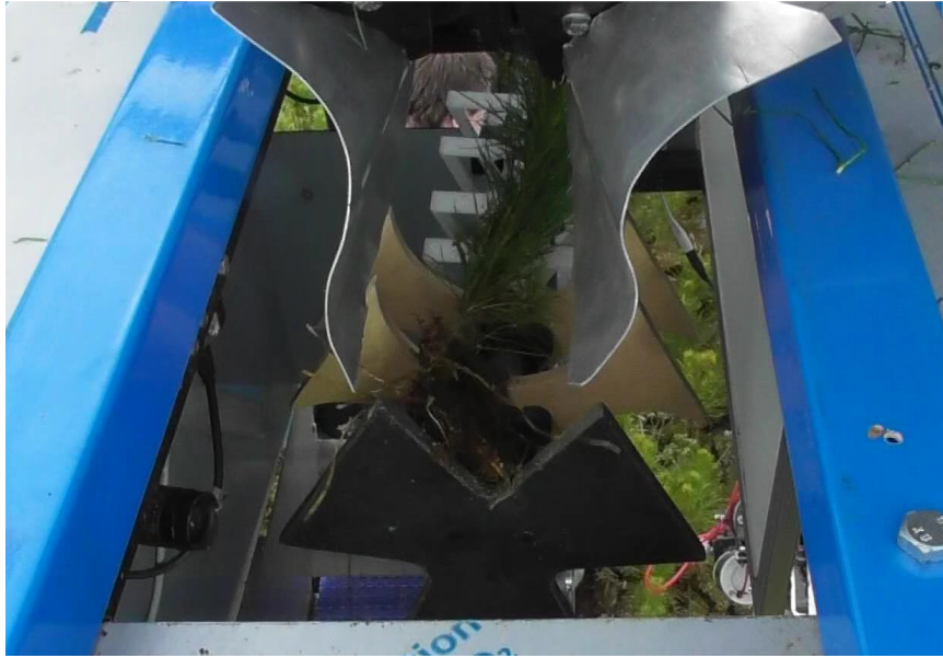
Figure 5.41: Tree failed transitioning into grading unit
