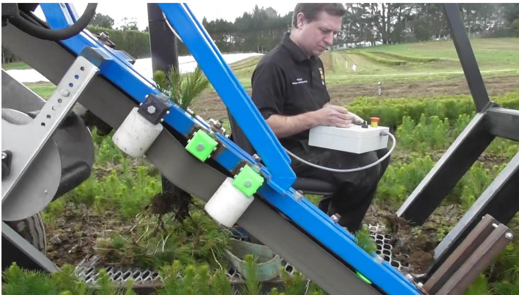
Figure 5.32: Operator steering and aligning belts with tree stock
