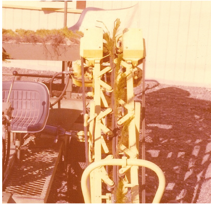
Figure 4.6: Lifter with sprung loaded idler pulleys [57]
