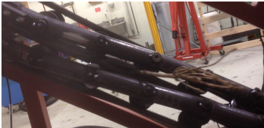
Figure 4.16: Reorientation of tree using twisted belts
