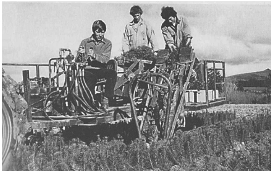
Figure 2.8: Single row lifter in use in New Zealand during the 1970s
