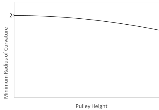
Figure 4.18: Minimum radius of curvature for tree in terms of pulley radius, based on pulley height
