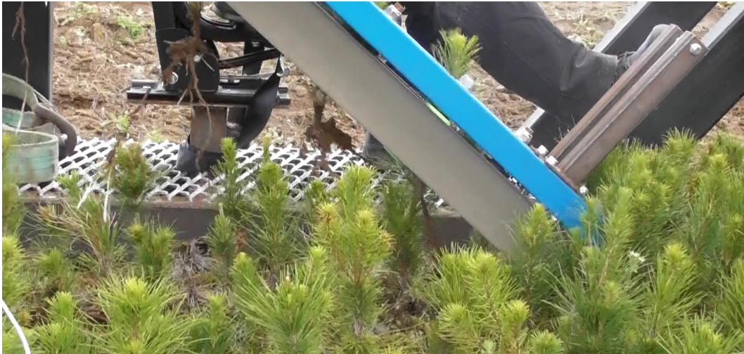
Figure 5.33: Lifting with the field factory
