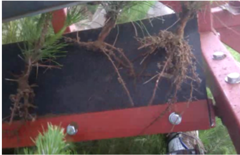
Figure 4.10: Oscillating rubber soil remover contacting roots
