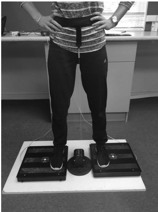
Figure 3 – Set up of the test session. Linear position transducer attached to a waist harness on top a force platform.
