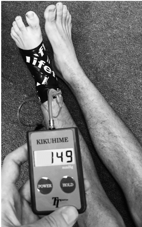
Figure 2 – The Kikuhime pressure monitoring device applied under the floss band.
