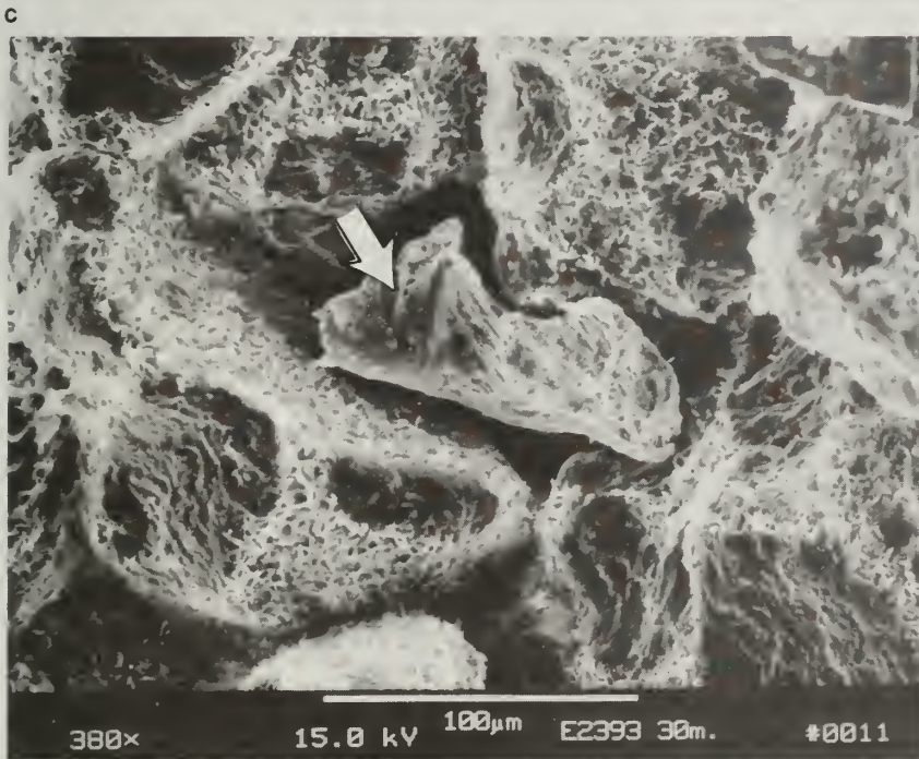
d c) An untreated sample (2,393.5-ft depth, Budmark 2 Morgan Coal) shows patchy calcite cement filling pores (arrows). This type of calcite is much more extensive than the minute late-stage crystals shown in figure 4a. Dissolution of this type of calcite would improve porosity and permeability of reservoirs. d) Partial dissolution of pore-filling calcite cement (arrow) after 30 minutes of soaking the sample (depth 2,393.5-ft, Budmark 2 Morgan Coal) in MCA. Compare this example with the untreated calcite cement shown in 4c. The edges of the calcite are etched and contrast sharply with the flat, smooth cleavage surfaces in the untreated sample. Note that the clay minerals appear to have been unaffected.
