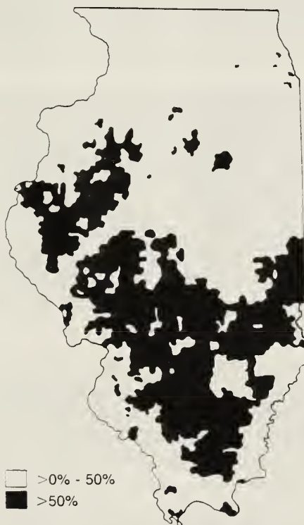
Figure 3 Areas of Illinois where more than 50 percent of the private wells are large-diameter dug or bored wells (NWWA 1986).
