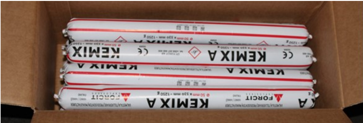
Figure 5.5: Kemix A emulsion cartridges ( \varnothing 50mm) used during production blasts.
