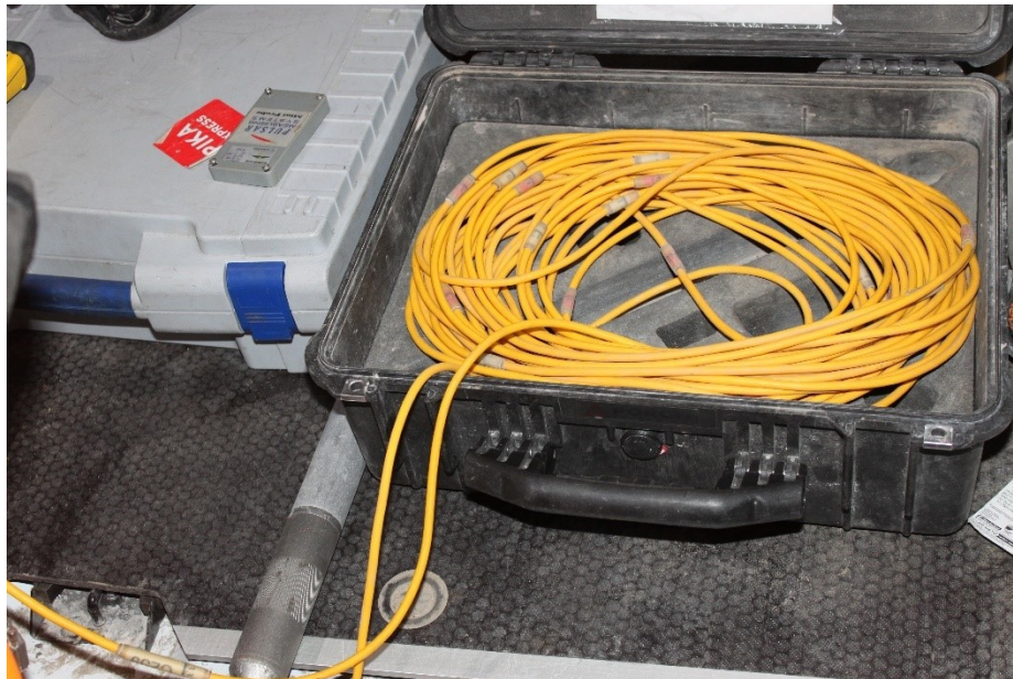
Figure 7.2: Drillhole deviation measurement probe and cable.
